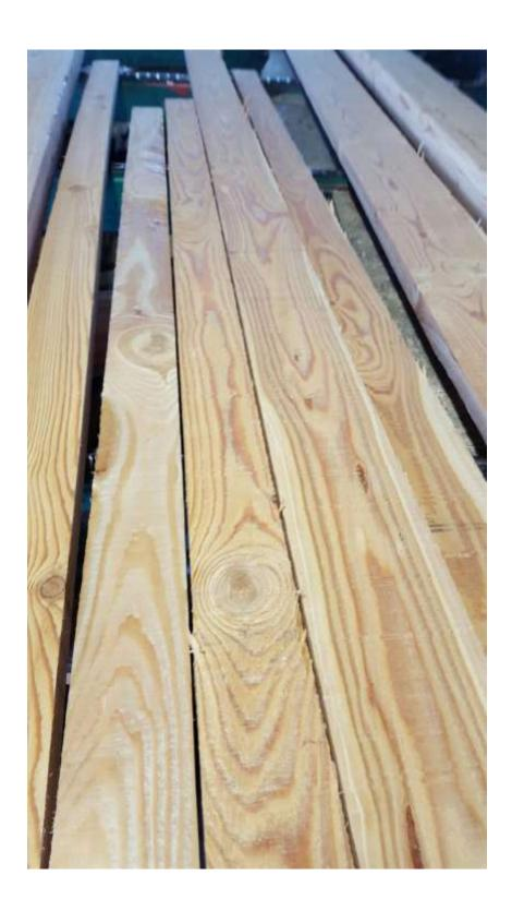
These three photos, also by Brian Parker, show the decking that was air dried over the winter. It went to 12%, with little drying degrade. It was so hard that inserting the moisture meter probe was difficult.
