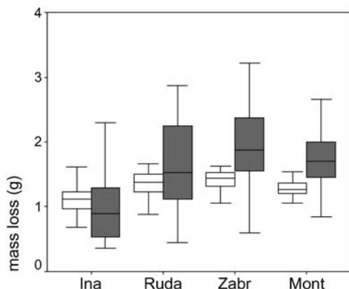
**Fig. 3** Mass loss observed within the investigated origins performing *Poria placenta* (white boxes) and *Coniophora puteana* (grey boxes) decay tests
